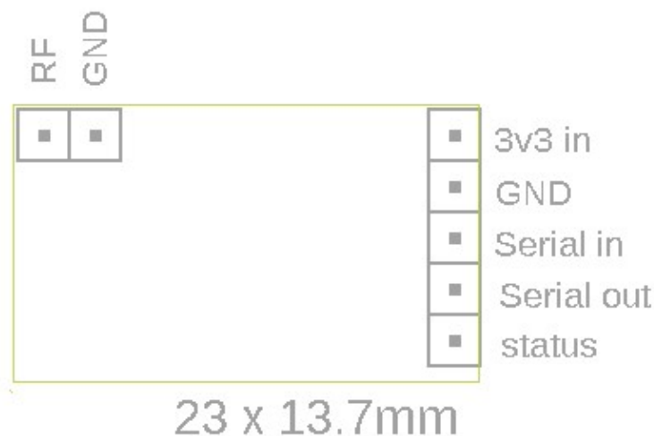
Figure 2: CWM2 Pinout and Dimensions
