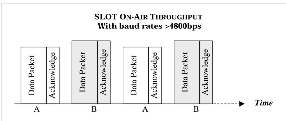
Figure 6: Two SpacePort Modem pairs operating Slot throughput
