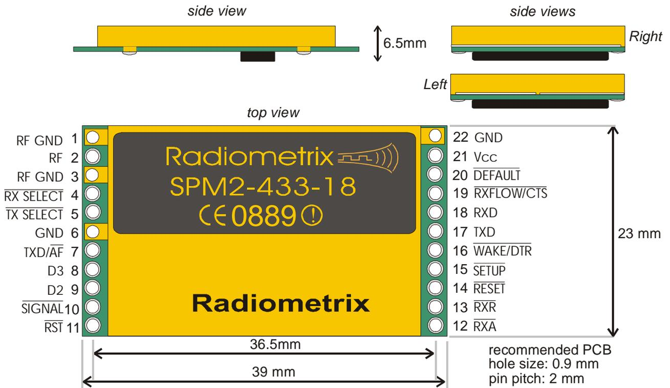
**Figure 2: Physical dimensions and pinouts**
