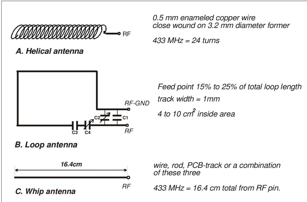
Figure 6: Antenna configuration
