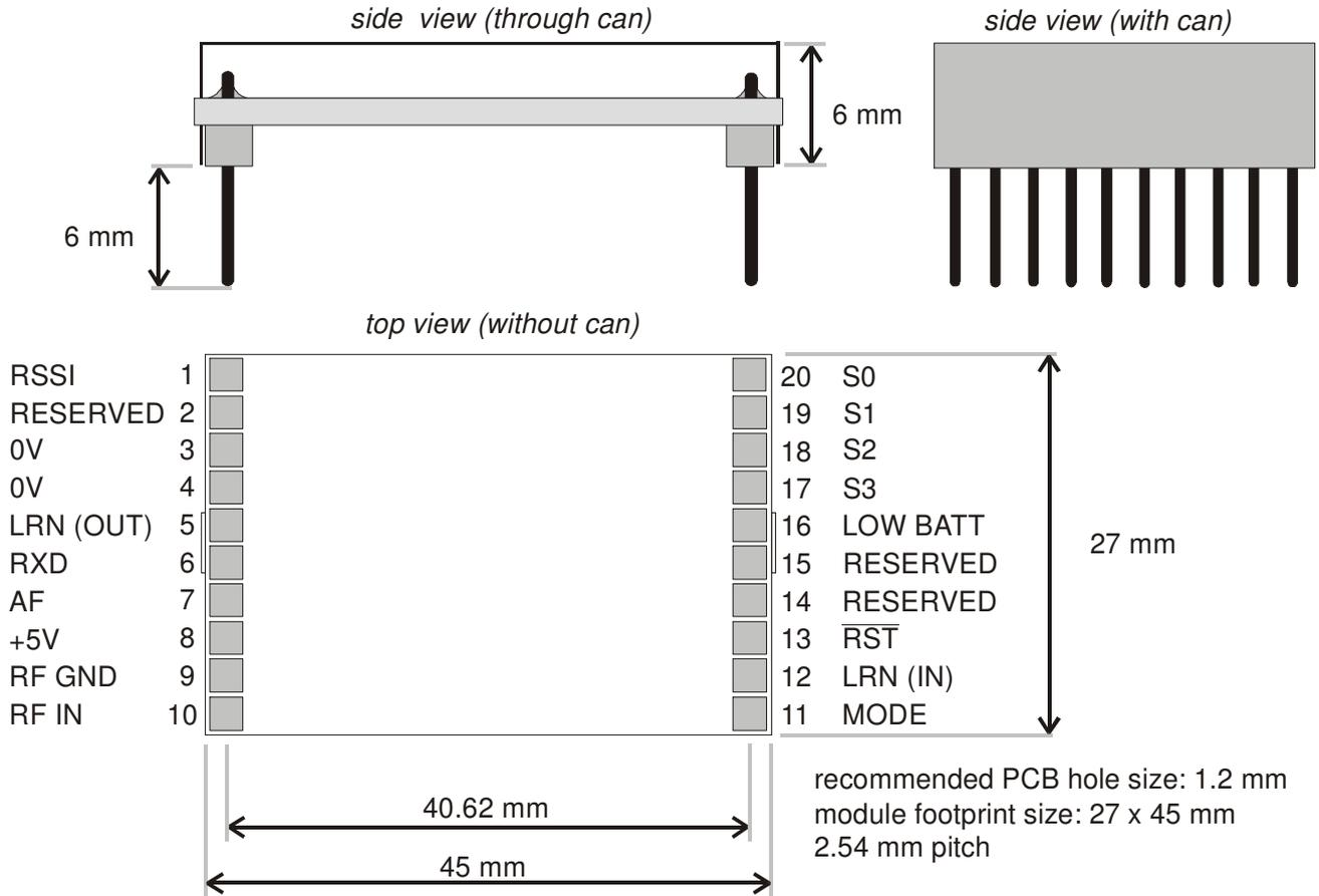
Figure 2: KRX2 Dimensions and pin-out
