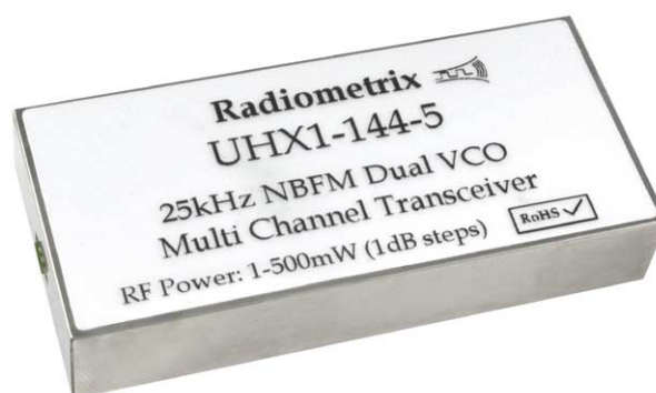
Fig 2: A 500mW multi channel VHF transceiver
