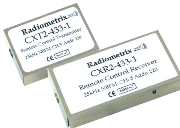
Figure 1: CXT2 transmitter and CXR2 receiver
